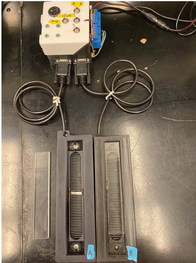
Fig. 1. The shuttle box apparatus with propeller controller in the upper left-hand corner. In this image, one of the plexiglass covers (A) has been removed so that the shock grid can be seen more easily. In the experiments, one cricket was placed into the compartment labeled A and one cricket was placed into the compartment labeled B. A piece of filter paper was placed under the left-hand side of the shuttle box to illustrate the midpoint for the two halves of the compartment. Once the cricket was inside the compartment, the plexiglass was placed over the compartment to ensure that the cricket maintained contact with the grid.
